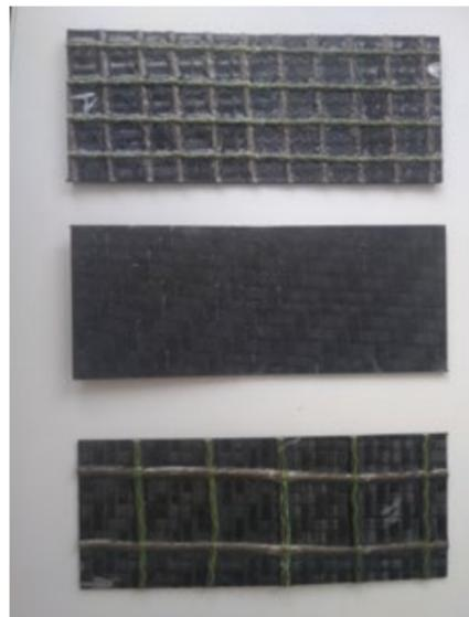
Key outcomes included the discovery that the use of PowerRibs increases the flexural strength and stiffness. The stiffness is increased by a factor 1.5 and the strength by a factor 1.3. The Team is considering which applications and components would be best suited to this material. The full report can be found in the appendix.
